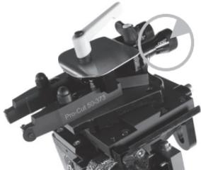
Turn the dials clockwise to advance the cutting tip depth. Each line on the dial indicates 0.0025"
