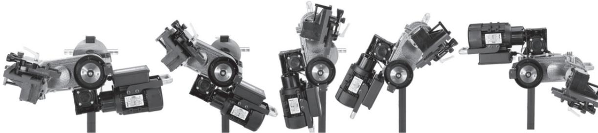
After loosening the trolley handle, the lathe can be flipped over to machine the opposite side of the vehicle.
