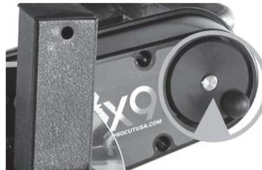
Move the cutting head by turning the knob shown above, clockwise for away from the rotor, counter-clockwise for towards the rotor.
