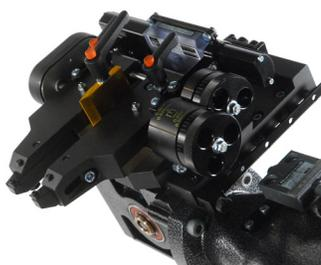
**G2X Cutting Head (50-1200)** slide, center, lock and set lock handles. Simple operation and visibility of the control knobs as they are facing the technician. This cutting head will also measure the thickness of the rotor before, during and after the cut.
