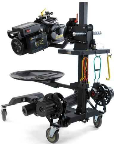
■ Pro-Cut's PFM 9.2DRO on-car brake lathe
