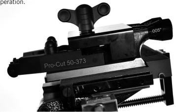
**NOTE** The Pro-Cut will mount right-side up on one side and upside down on the other. Always start right-side up; this way, when you proceed to the other side of the vehicle, the offset of the cutting head will already be set, with the cutting head firmly in the dovetail. Never attempt to move the cutting head laterally with the lathe upside down.
