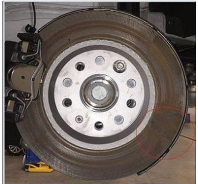
Figure 8: Corrosion, brake pad stuck to brake disc.
