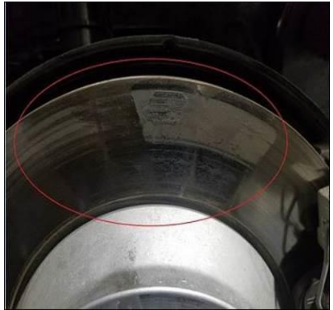
Figure 10: Brake Pad stuck to Brake Disc.
