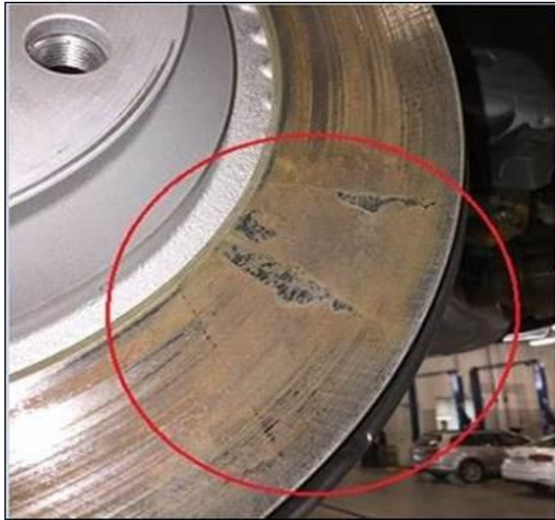
Figure 7: Corrosion, brake pad stuck to brake disc.
