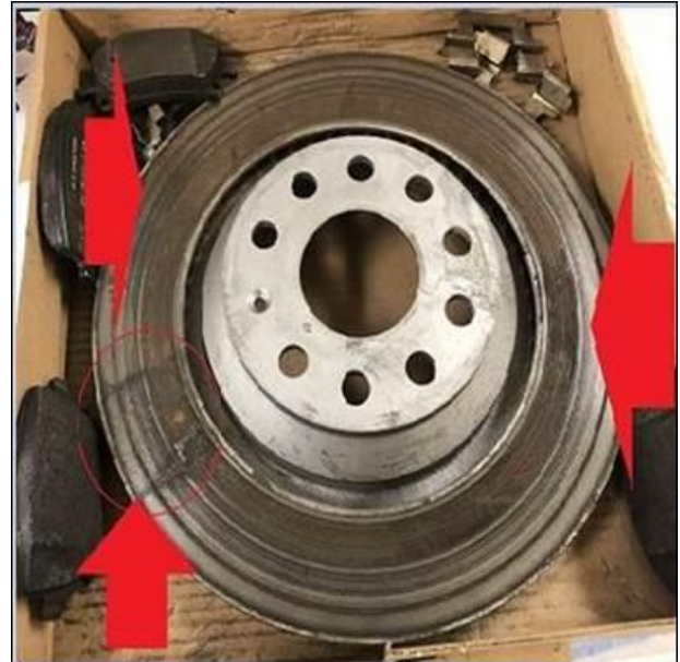
Figure 6: Corrosion, brake pad stuck to brake disc.
