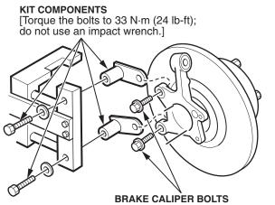
**BRAKE CALIPER BOLTS** [Torque to 54 N·m (40 lb-ft); do not use an impact wrench.]
