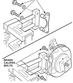
[Torque to 54 N·m (40 lb-ft); do not use an impact wrench.]
