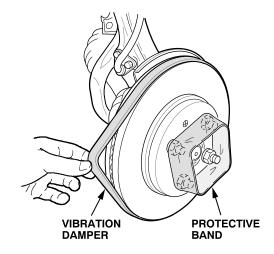
If you are not using the power drive system, use a fabric tie-down strap to secure the brake disc that is opposite to the one you are refinishing. If you are working on a Prelude with ATTS, do not use a tie-down strap; let both wheels turn freely.
