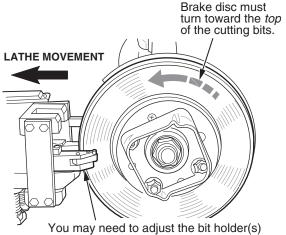
for proper cutting of the brake disc.
