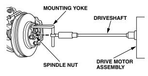
Set the lower toggle switch on the drive motor assembly to FWD (counterclockwise rotation) or REV (clockwise rotation).
