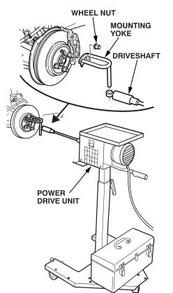
3. Attach the driveshaft on the drive motor assembly to the mounting yoke, making sure the center line of the driveshaft is level with the spindle nut on the wheel hub.
