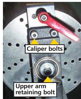
◀ View from the operator's side reveals there are 2 caliper bolts requiring the use of a 4mm Allen to secure. They are also knurled, so for demo purposes they can be finger-tightened for ease of assembly. The upper trolley arm post through the 2 bearings is secured with 1- 6mm Allen bolt that is also knurled for easy assembly during demo service.
