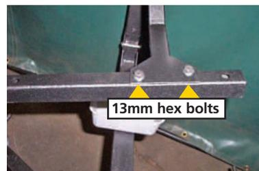
◀ Note that the bolts that secure the cross piece to the upper trolley arm are now a 13mm hex style vs. the old 6mm Allen.
