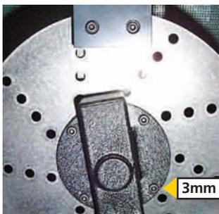
◀ The lathe side of the trolley reveals the 4- 3mm Allen bolts that secure the disc to the upper trolley arm. These bolts screw into 4- 7mm nylon locking hex nuts.
