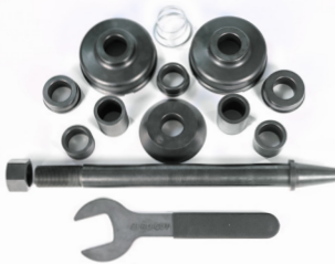
50-4260 1 7/8ths HD Arbor Kit Includes: 5.5" cone, 6.5" cups, spring, wrench, and spacers
