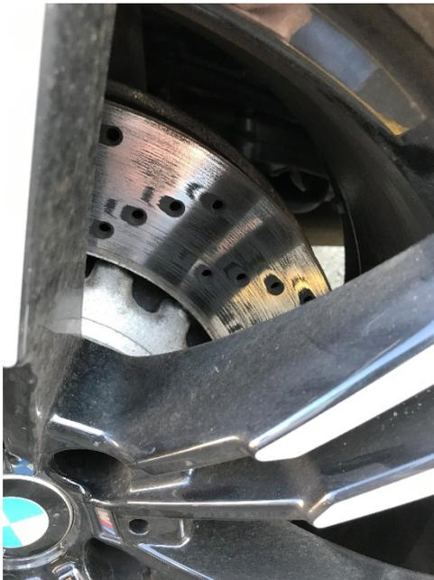
The customer should be made aware that the trailing marks will become more visible with brake applications and will eventually disappear with normal driving.
