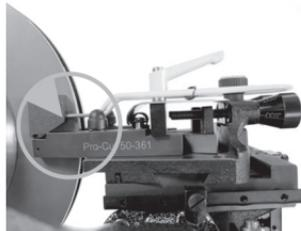
The chip deflector rides over the cutting arms as shown above. The chip deflector should be used every time. **Guard not shown for clarity.**
