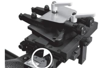
Note the Automatic Shut-Off Switch Above. The shut-off cam will depress the stop button when the cutting tips clear the rotor.
