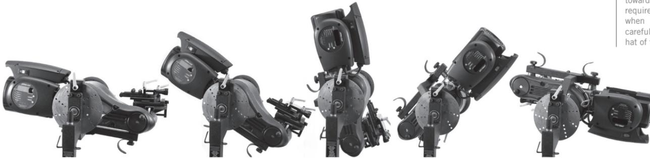
After loosening the trolley handle, the lathe can be flipped over to machine the opposite side of the vehicle.
