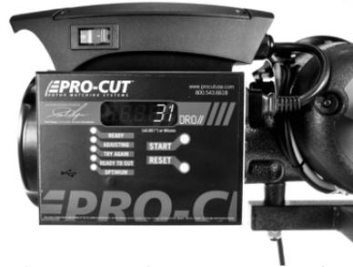
This value represents the average compensation time recorded in seconds over the life of the lathe.
