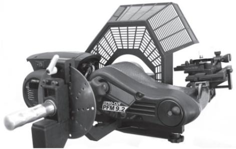
FIG:1 Lathe in upright position. Note that adjustments to cutting head are simpler in this position.
