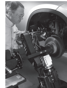
Step 2: Technician mounts the lathe to the adapter
