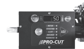
DRO computer in READY mode displaying speed.
