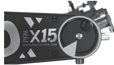
Move the cutting head by turning the clutch knob shown above, clockwise for away from the rotor, counter-clockwise for towards the rotor.
