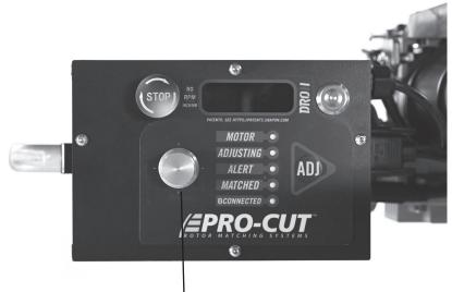
Press the control knob to enter Set-up mode.
