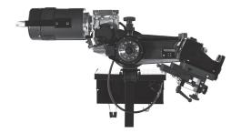
Lathe in upside-down position. You will need to flip the lathe over into this position to machine one side of the vehicle if there is a dust shield, or other interference behind the rotor.
