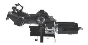
$\Box$  Lathe in upright position. Note that adjustments to cutting head are made in this position.
