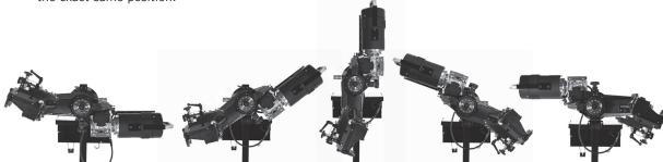
After loosening the trolley handle, always rotate the lathe by the motor to avoid cord wrapping / tangling to machine the opposite side of the vehicle.
