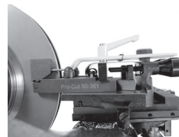
The chip deflector reduces vibration.
