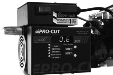
| This display of final compensation equals .0006"
