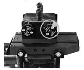
Turn the dials clockwise to advance the cutting tip depth. Each click of the dial indicates .001".
