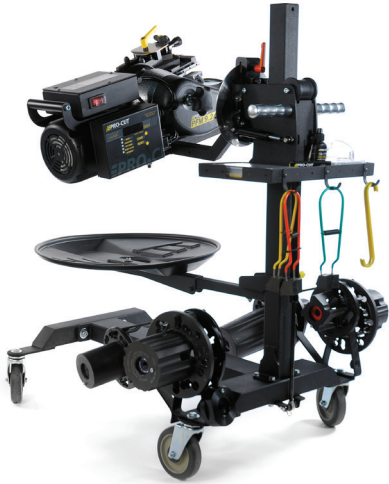
■ Pro-Cut's PFM 9.2DRO on-car brake lathe
