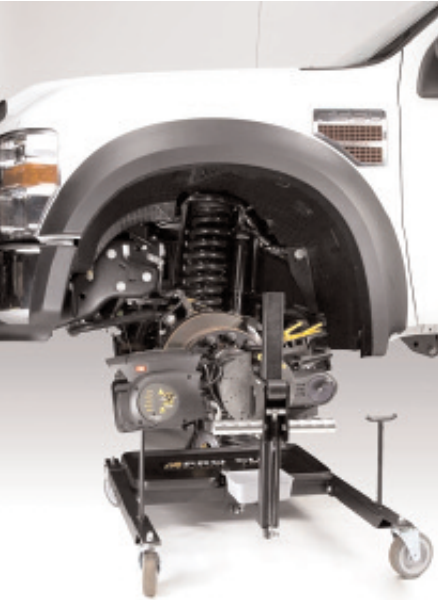
Pro-Cut's PFM 9.2SL with Low-Boy Trolley machining a F-550 SuperDuty truck.
