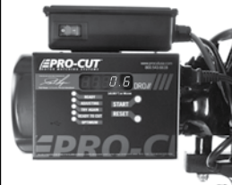
DRO computer compensated for lateral run-out to 0.0006" and ready to cut.
