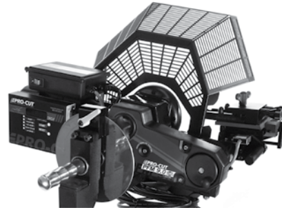
FIG:2 | Lathe from different direction. You will need to flip the lathe over to machine one side of the vehicle if there is a dust shield, or other interference behind the rotor.
