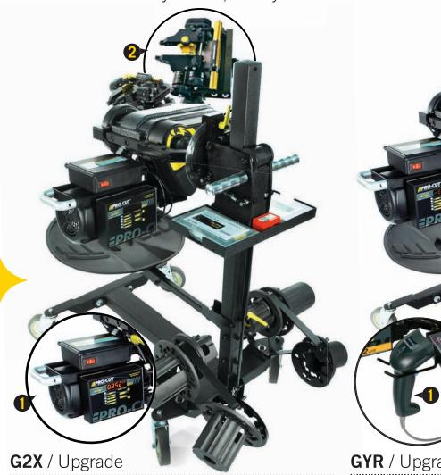
Upgrade your DRO lathe and get live digital read-out of rotor thickness! The "SMART" cutting head has increased mass, parallel cutting arms, linear transducer and over-sized face-mounted dials. The custom application turns the lathe cutting head into a live micrometer with rotor thickness shown in inches or millimeters on the LED display. You'll never lose this micrometer!
