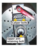
✓ View from the operator's side reveals there are 2 caliper bolts requiring the use of a 4mm Allen to secure. They are also knurled, so for demo purposes they can be finger-tightened for ease of assembly. The upper trolley arm post through the 2 bearings is secured with 1- 6mm Allen bolt that is also knurled for easy assembly during demo service.
