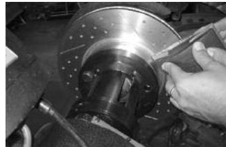
Upon cutting rotors, sand for 1 minute per side with 150 grit sandpaper and wash down with soap and water.
