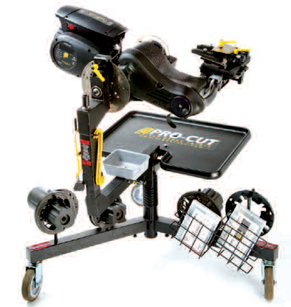
Pro-Cut's latest model — the PFM 9.2 DRO-Live On-Car Brake Lathe
