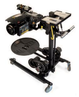
**GYR Compatible Rotor Matching System.** The innovative data system captures critical brake geometry, confirming the quality of every brake repair. The full GYR on-car brake lathe will become an Essential Tool for Honda Canada in 2011.
