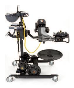
**GYR.** Pro-Cut's new complete brake repair system directs techs through the rotor matching process and captures the finished condition of each serviced rotor.
