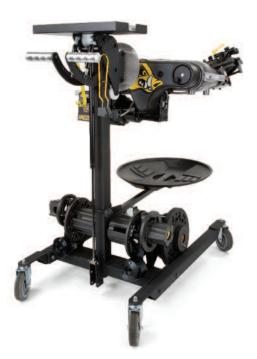
Warthog. Pro-Cut's latest rotor matching system merges platform, design, and technology to create a machine of unprecedented ruggedness and versatility. The Warthog can service virtually any rotor on any lift.
